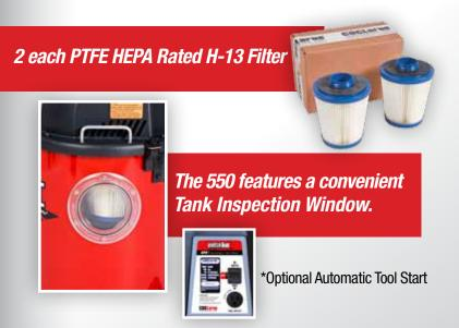
Model PB-550 (P/N# 103550) is a High-Efficiency Particulate Air Vacuum with a filter fractional efficiency rating of 98.0% @ .3 micron at a CFM flow rate up to 140. The 550 model comes standard with two HEPA H-13 filters, Pulse-Bac® Technology, our Cyclonic Debris Management system, a 8 gallon powder coated tank, 15' x 1.5" crush proof self locking vacuum hose and a tank inspection window. An optional \*automatic tool start is also available.
