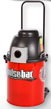
Model PB-575 (P/N# 103575) is a High-Efficiency Particulate Air Vacuum with a filter fractional efficiency rating of 98.0% @ .3 micron at a CFM flow rate up to 140. The 575 model comes standard with two HEPA H-13 filters, Pulse-Bac® Technology, our Cyclonic Debris Management system, a 8 gallon powder coated tank, 15' x 1.5" crush proof self locking vacuum hose and a tank inspection window. An optional \*automatic tool start is also available.
